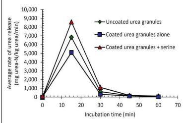
Comparison of urea release rates over time for coated and uncoated fertilizers. Green: Uncoated fertilizer; Blue: Fertilizer with aptamer-containing coating in the absence of any target in sand; Red: Fertilizer with aptamer-containing coating in the presence of the target molecule serine in sand.
