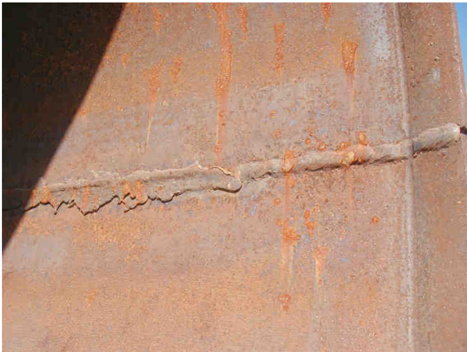
Figure W2: Welding inconsistency on the inside of a poorly welded tank. Note the inconsistent finish on the weld and poor penetration on the far right end of the weld.
