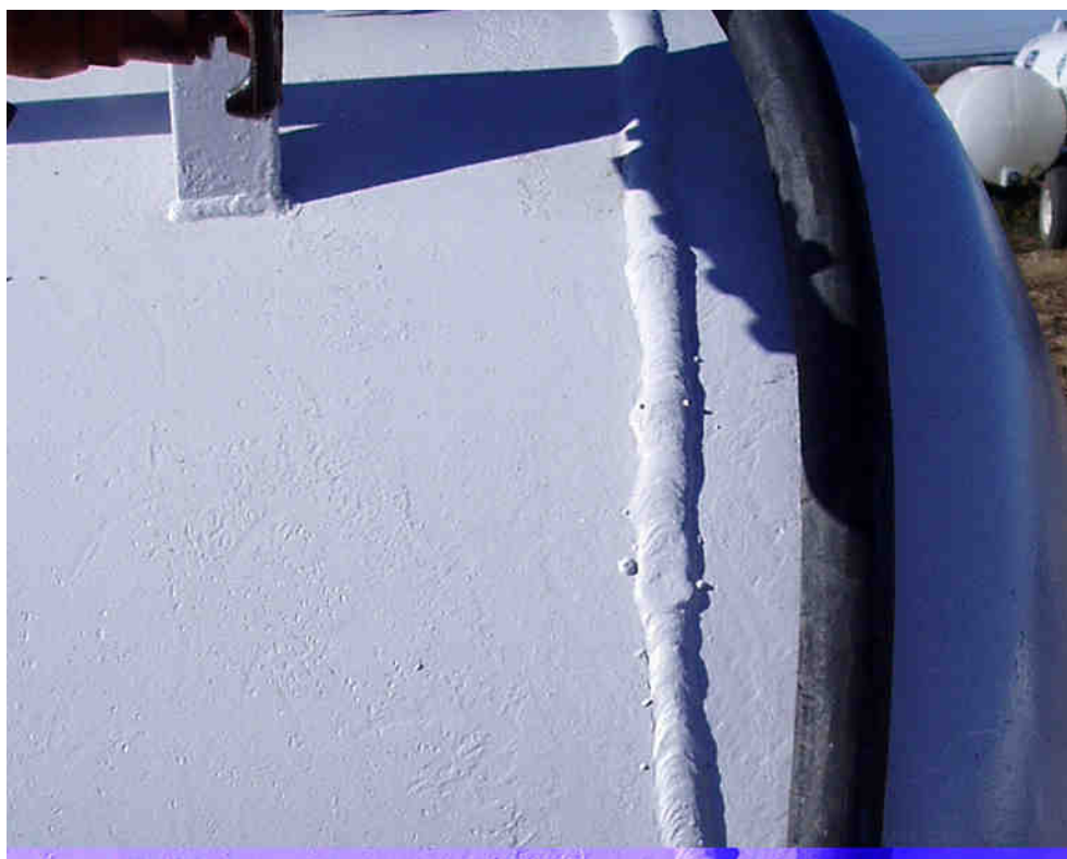
Figure W4: Close up of illegal weld on tank head.
