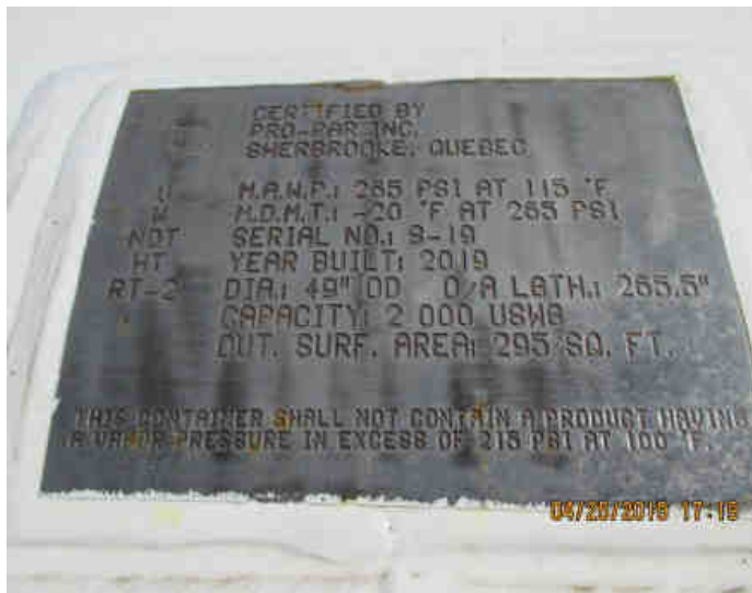
Figure 12.1 b.) An example of a manufacturer's data plate on a TC51 tank
