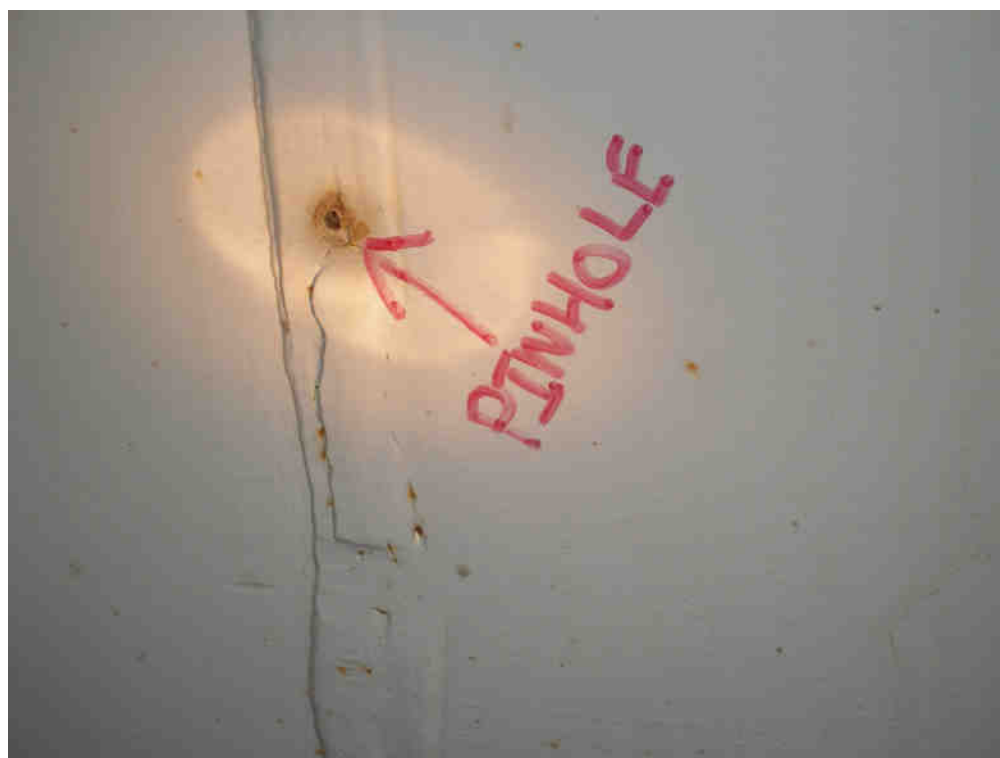
Figure W8: Poor weld with pinhole leak.
