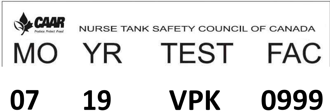
Figure 13.2 Example of a B620-20 marking indicating the performance of an External Visual Inspection and a Hydrostatic Pressure Test. The test was conducted in July, 2019 by a facility with the last four (4) digits of their Transport Canada registration number being 999.
