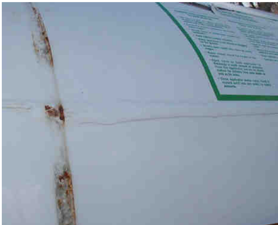
Figure W10: Poor welding example with varying weld width.
