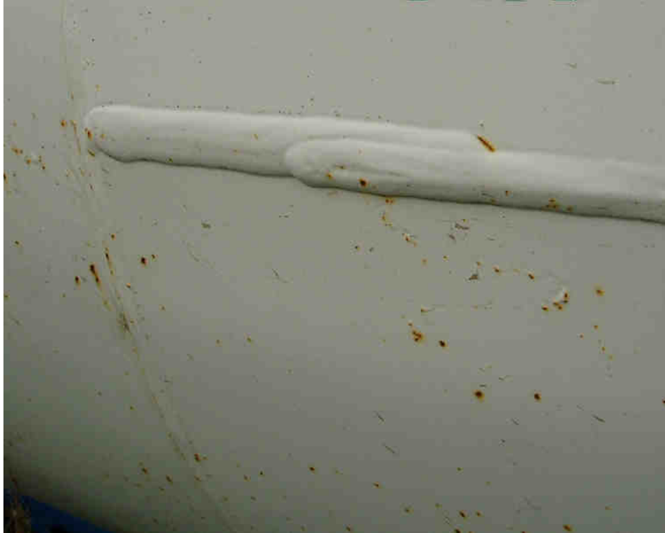
Figure W5: Inappropriately lapped weld.
