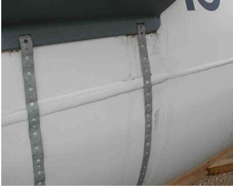
Figure W11: Poor welding example with varying weld width.
