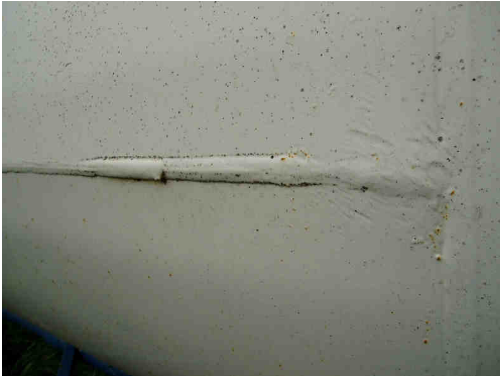
Figure W9: Poor welding example with varying weld height and width and a long overlap.
