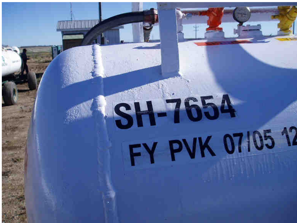
Figure W3: Illegal weld on head of tank. Tank head had been removed and welded back on.
