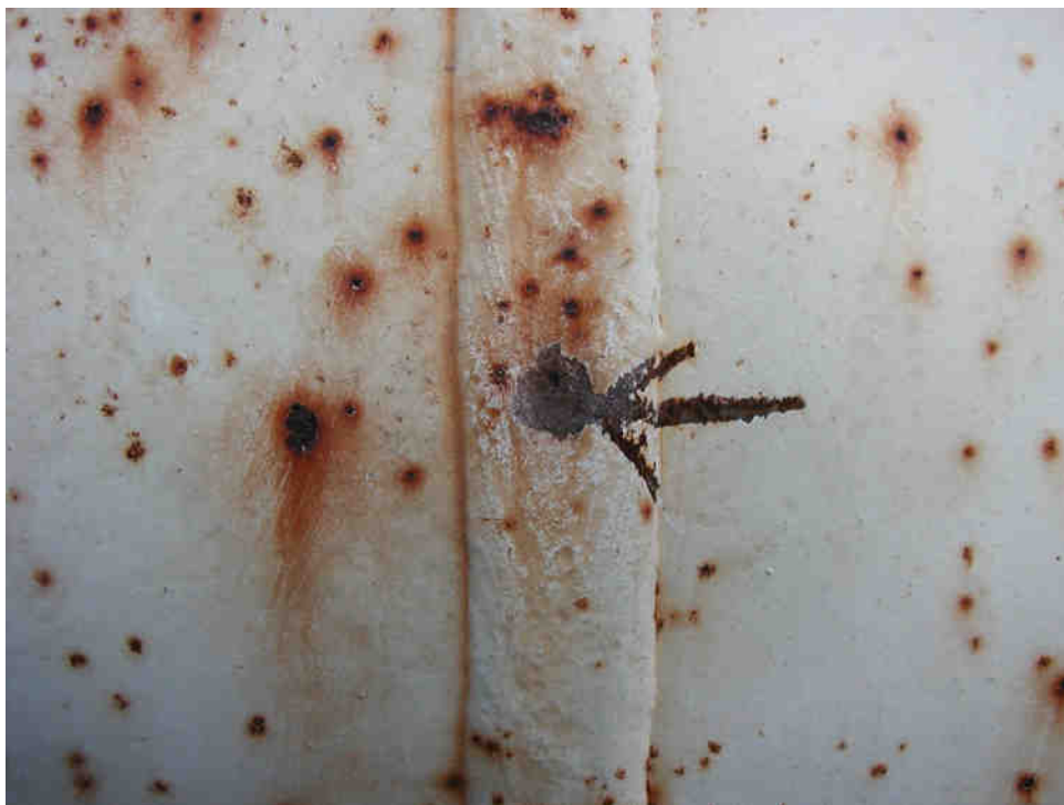
Figure W6: Pinhole leak in head to shell weld.
