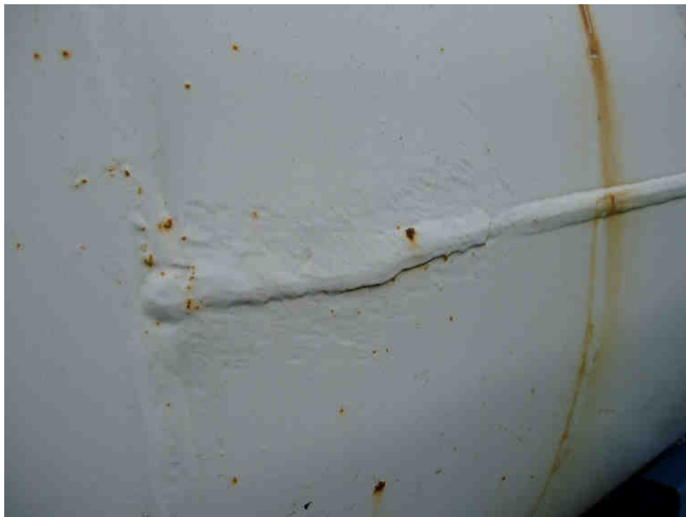
Figure W12: Poor attempt at repair where tank and weld have clearly been worked.
