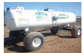
Figure 12.2 Side view of an anhydrous ammonia nurse tank
