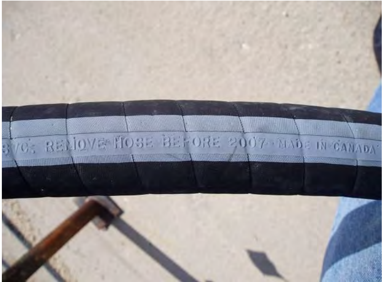
Figure 8. Hoses Marked for Remove from Service Date
