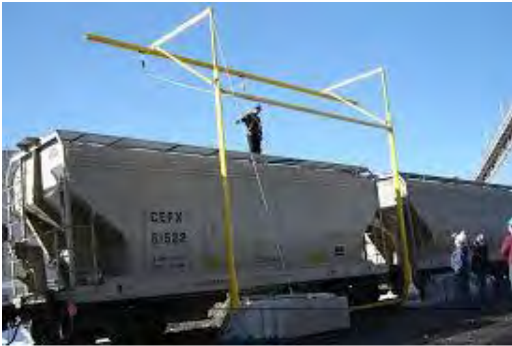
Figure 6. Example Fall Arrest with Engineered Tie-Off System
