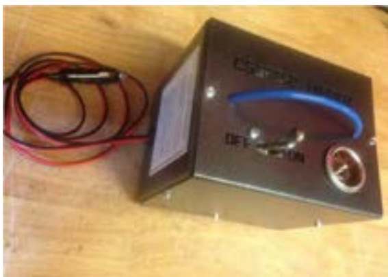
Figure 1: Example of a manual airbox link for remote shut off
