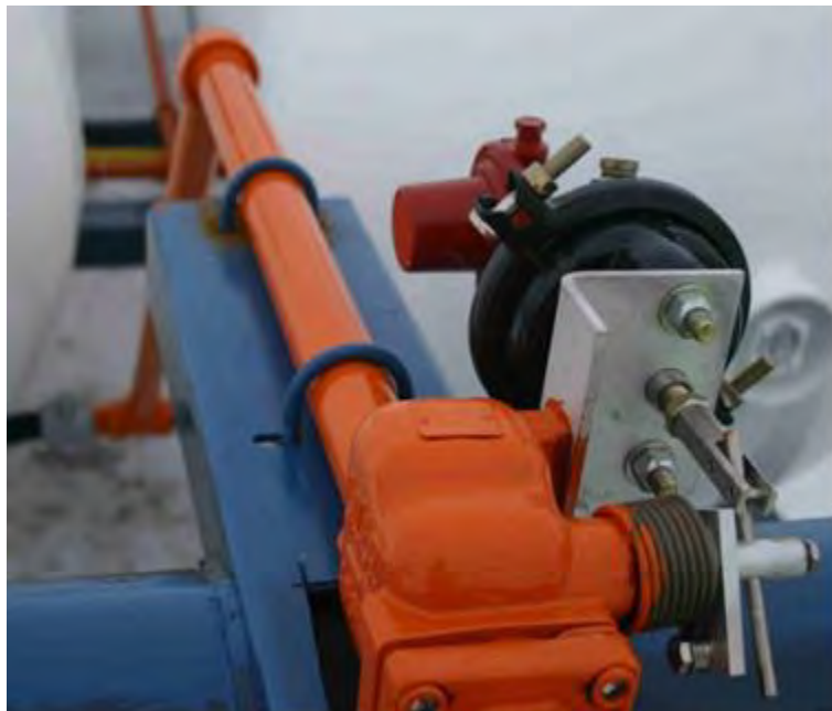
Figure 2: Example of a shut down system installed on a tank
